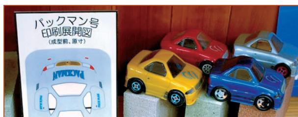
Completed by printing a development view on PET materials and vacuum forming
